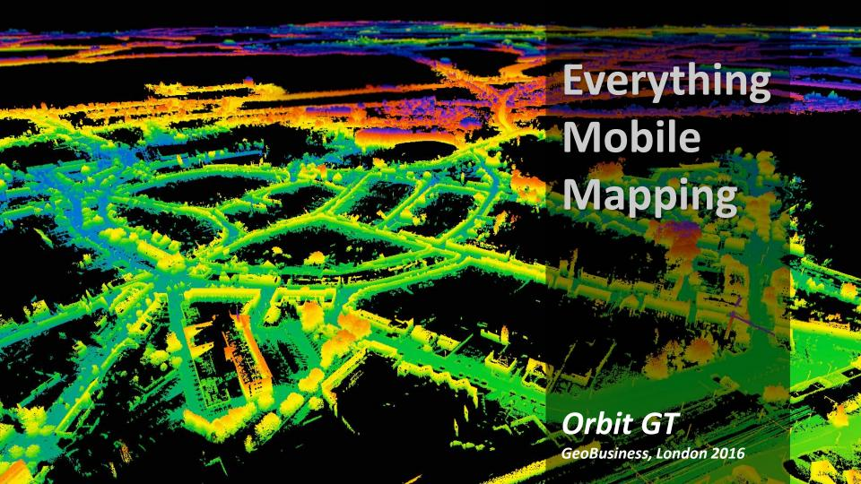
Mobile Mapping brings the full representation of 3D reality onto the desktop, using sensors mounted on a mobile vehicle (car, train, boat, bike, uav, even a person).
